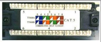
The photo above shows part of the back side of a typical category 5E patch panel. The method of connection is by insulation displacing '110' blocks. Note the connection diagram, showing connection for both 568A and 568B wiring schemes.
